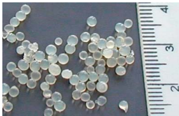
Figure 9 Beads produced from Ca-alginate and TEOS containing co-encapsulated F_{\text{ate}}\text{DH} , F_{\text{ald}}\text{DH} , and ADH.
